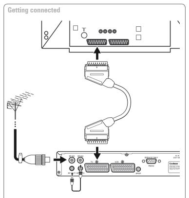
Connect the cable that comes from your aerial to the RF IN socket on the back of your Freeview+ digital TV recorder.
